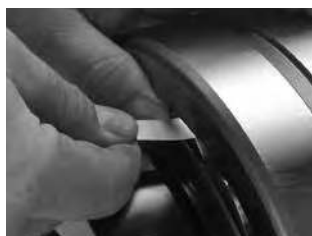
Fig. 14. Measure RIC before installation.
