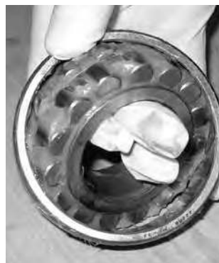
Fig. 21. Grease can easily be packed by hand.
