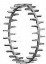
Fig. 5. EM/YM One-piece, machined-brass, roller-riding, finger-type cage.
