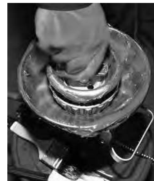
Fig. 22. Mechanical grease packer.
