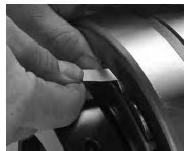
Fig. 18. Measure RIC before installation.
